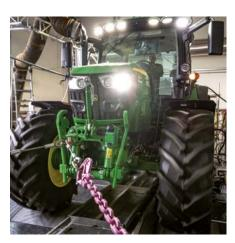
The PowerMix test is made up of 14 test cycles which simulate various loads on the tractor while measuring its fuel and AdBlue consumption, power output and efficiency.
