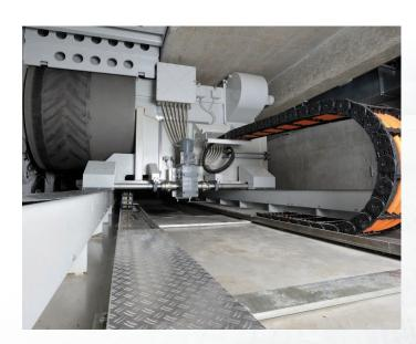
All inputs and outputs measured can be recorded. The recordings comprise fuel input, actual wheel payload, pto and hydraulic output as well as exhaust emissions on vehicles of up to 700kW ( $\approx$  1,000hp). The testbed also measures the efficiency of electric drivelines on electric and hybrid vehicles.
